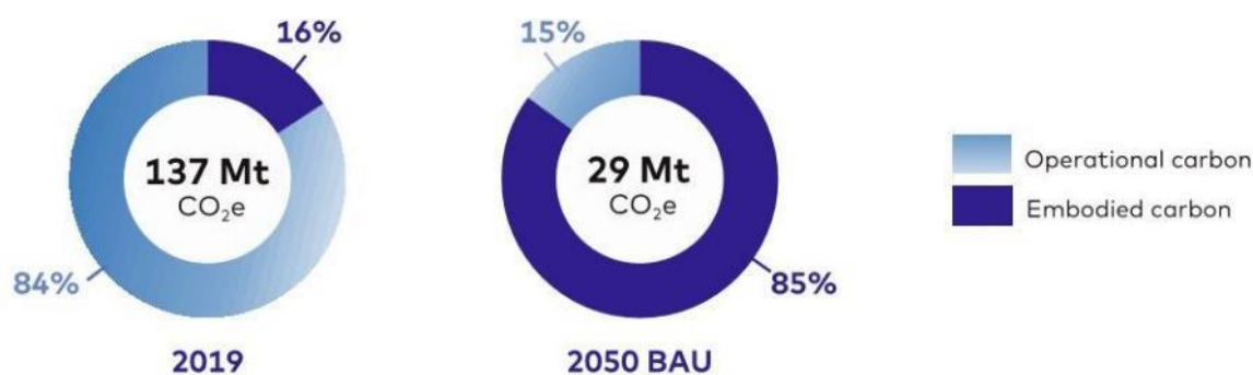
Figure 2: Future estimates for carbon emissions from Australian building stock show embodied carbon dominating emissions. Sourced from GBCA and thinkstep-anz. (2021). Embodied Carbon and Embodied Energy in Australia's Buildings.
